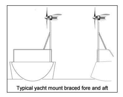
For inland watercraft such as narrow boats, a hinge-down tower arrangement can be utilised to allow for rapid lowering of the turbine for passage under low bridges etc.
